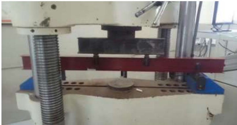
Test set up of I beam
